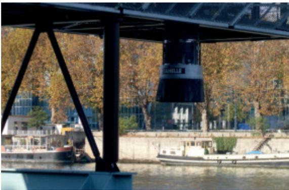
The Stanelle JET loaders TYPE **RONDO 350 / 400 / 500** with an extended hub are designed for loading ships and slagheaps. The required volume of exhaust air of approx. 2,000 - 3,000m<sup>3</sup>/h can be extracted via the suction nozzles by using an appropriate dedusting unit.
