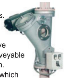
The **ZD accessory nozzle** is used for conveying lines of high pressure conveying plants. It is installed mainly behind the pressure vessel in order to ensure a lean phase conveying. The ring-gap-nozzle can also be used within the conveying line e.g. at the riser tube.
